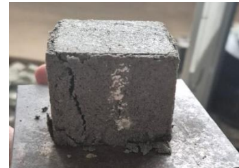
Fig. 7. Shear failure of the graphene-enhanced mortar cube after compression test
