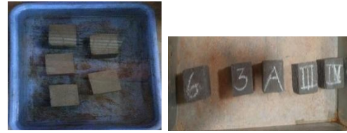
Fig. 9. Graphene oxide mortar cubes in the water bath and cubes after been placed in oven
