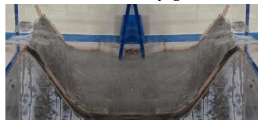
Fig. 11. Casting of scaled model of canal cross section with graphene enhanced mortar for seepage test
